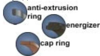
The assembly is composed of a self lubricating, wear resistant cap ring, made from bronze filled PTFE, and a NBR energizer. Thermoplastic split anti-extrusion rings support the seal on both sides and prevent contamination of the energizer and cap ring. These seals are designed to be used in a variety of equipment and are well suited for the heavy duty and high friction environments of earth moving and other off-highway equipment.
